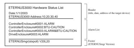
The "alarm history messages" shown above indicate the status results obtained from the target device. The following message is output when all components of the target device are normal.
